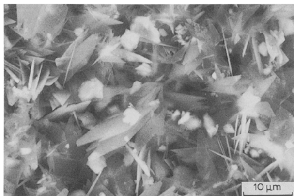
Figure 3 The products formed in the first 15 min of reaction at a \text{Ca}(\text{OH})_2/\text{HAp} ratio of 1.
